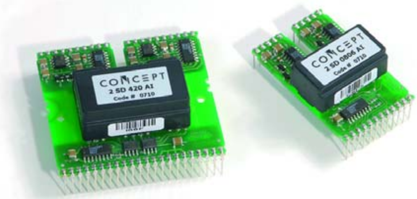
Figure 4: Dual-channel IGBT driver cores with external n-type DMOS driver stages for 20A / 4W gate capability (left), and a fully integrated version for 5.5A / 0.8W gate capability (right).
