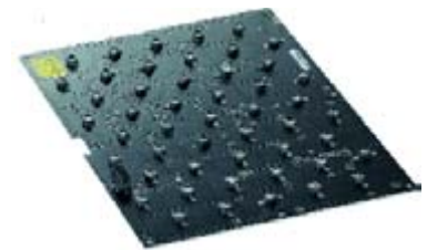
Figure 6: LED Boards: HB LEDs mounted onto Metal Core PCB
