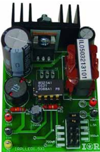
Figure 4: The IRS2540 and its sibling, the IRS2541, support bus voltages as large as 200 and 600 V, respectively.
