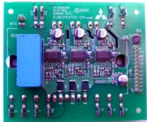
Figure 2: Evaluation Board for 1200V DIP-CIB (EVBCP25TD1-24A) (1200V HVICs, Shunts, bootstrap circuit and a driver for the brake)
